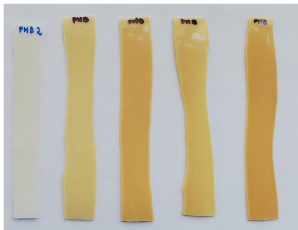
Fig. 1. Samples of polyhydroxybutyrate (PHB) before and after 100 h, 200 h, 300 h and 400 h of the thermooxidative aging process at the temperature of 100°C.
